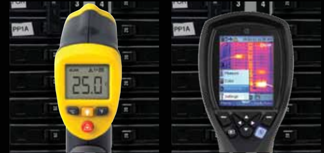
Spot pyrometer, temperature measurement in one spot.
